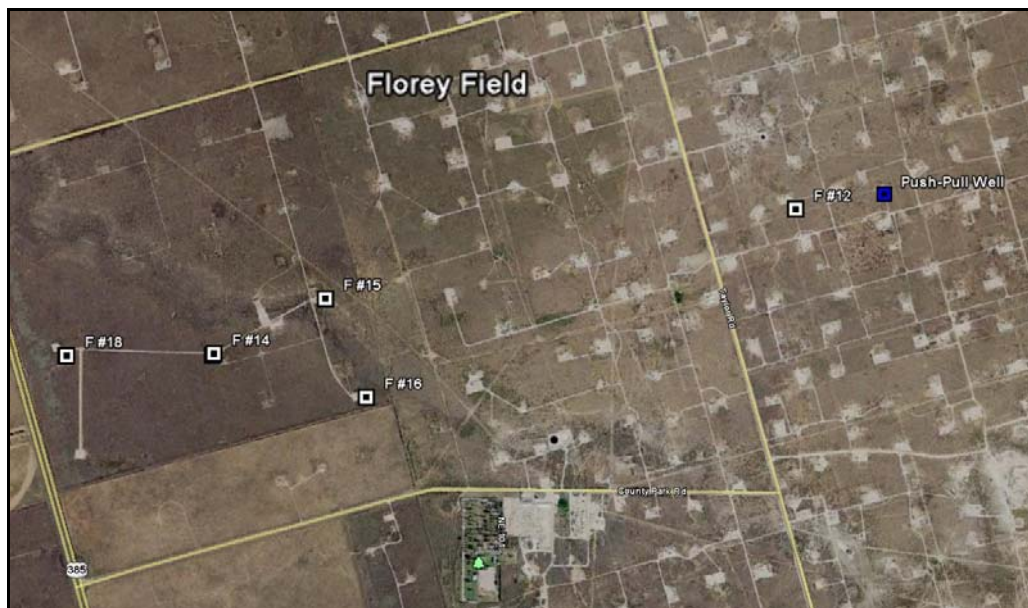
Figure 5: Google Earth image of the Florey well field, located approximately 10 miles north of Andrews, Texas. The locations of the experimental push-pull well and the injection source water well (F #12) are shown.
